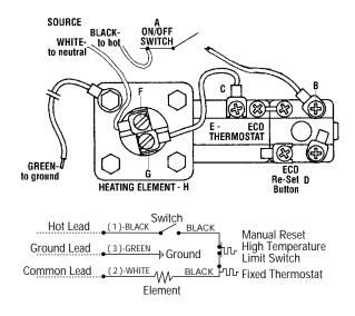
Early model water heaters with 110 VAC heating capacity used a bolt-on heating element and a one piece thermostat/E.C.O..
