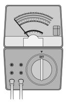
**Circuit Board Tester** - The tester is capable of testing any of the circuit boards (Fenwal and Channel models) that we have used on our water heaters. It is a simple table top device that will diagnose the following items on a circuit board: power circuit, sense circuit, spark generation and the lock-out mode. For use on circuit boards with a flying lead connection, splice a wire into the black wire of the tester harness with a 1/4<sup>°</sup> male terminal on the free end.
