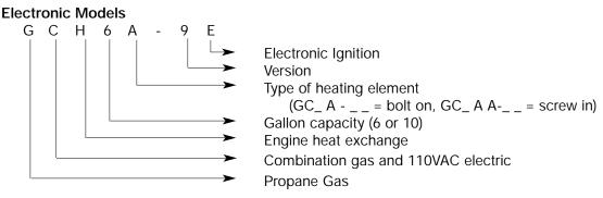
**NOTE:** When replacing the element on a combination gas/110 VAC unit, always check the back of the heater for the type of element it has. It will either be a bolt-on or screw-in element. They are not interchangeable.
