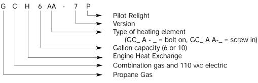
**NOTE:** When replacing the element on a combination gas/110 VAC unit, always check the back of the heater for the type of element it has. It will either be a bolt-on or screw-in element. They are no interchangeable.
